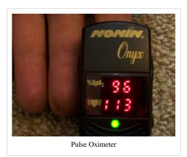
of the red and infrared light caused by the difference in color between oxygen-bound (bright red) and oxygen-unbound (dark red or blue, in severe cases) blood hemoglobin, a measure of oxygenation (the per cent of hemoglobin molecules bound with oxygen molecules) can be made.
